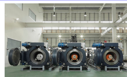
超臨界CO 2 染色(ColorDry)装置, (Sole Collector News (2013)HPより)
