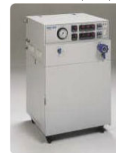
超臨界CO 2 染色(ColorDry)装置, (Sole Collector News (2013)HPより)
