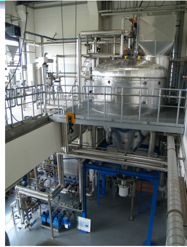
PGSS™/CPF™ plant Fraunhofer Institute UMSICHT (Germany) 150/300 kg/h, up to 35 MPa
