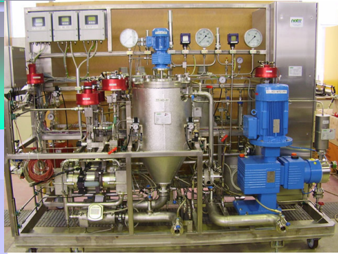
PGSS™/CPF™ plant Food industry (Germany) 40/80 kg/h, up to 35 MPa
