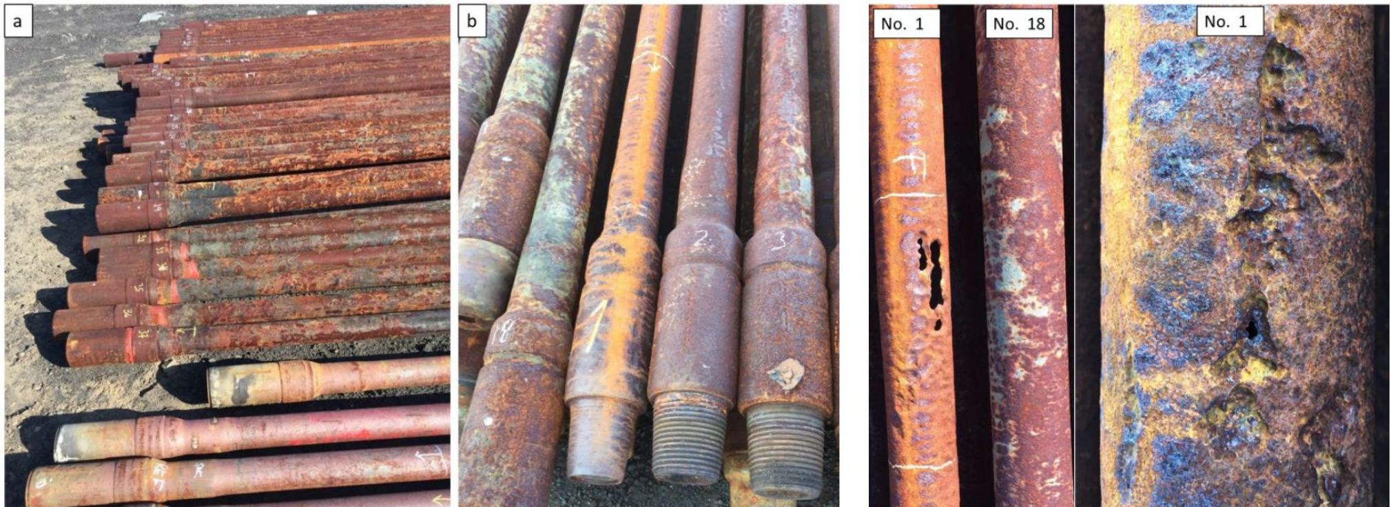
The injection pipe sections from different depth of the IDDP-2 well as well as un-used drill pipes for comparison (bottom of the photo).
